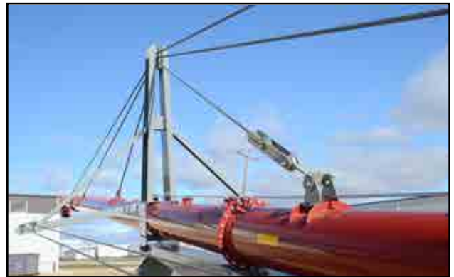
Fig 13 - Auger 14 truss system
