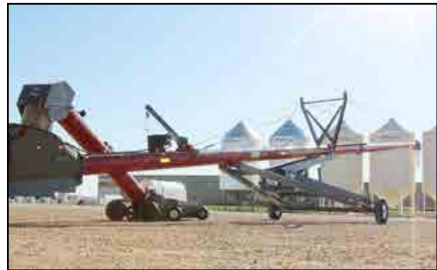
Fig 16 - Auger in fully collapsed position
